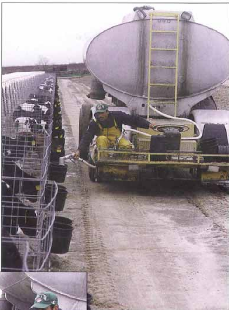
This ingenious calf feeding truck was conceived of at Joseph Gallo Farms and custom-built by a local fabricator. The chassis and rolling gear were salvaged from a TMR feed truck, and a 2,000-gallon milk tank is mounted to the frame. The hydraulic steering gear and driving position have been radically repositioned to allow driver Armando Arroyo to fill each calves' buckets in gas pump fashion, in just three seconds each, as he slowly idles by and without ever leaving his seat.
