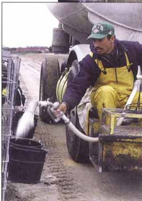
This ingenious calf feeding truck was conceived of at Joseph Gallo Farms and custom-built by a local fabricator. The chassis and rolling gear were salvaged from a TMR feed truck, and a 2,000-gallon milk tank is mounted to the frame. The hydraulic steering gear and driving position have been radically repositioned to allow driver Armando Arroyo to fill each calves' buckets in gas pump fashion, in just three seconds each, as he slowly idles by and without ever leaving his seat.
